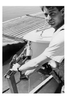
Reach into the boat from the dock, <u>release the keel</u> <u>lift line</u> and then <u>slowly</u> lower the keel. This will stabilize the boat. <u>Remove the "rudder lock" pin</u> out of the rudder, lower the rudder blade all the way down to vertical, and then <u>re-insert the "rudder</u>
