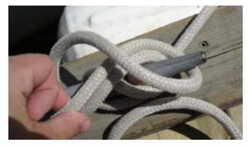
Step 4: Once you have done the loop, pull on the painter in order to tighten it and voilà! You have tied your boat to the dock! Check that the lines lies smoothly on itself and makes a neat, snug fit on the cleat.
