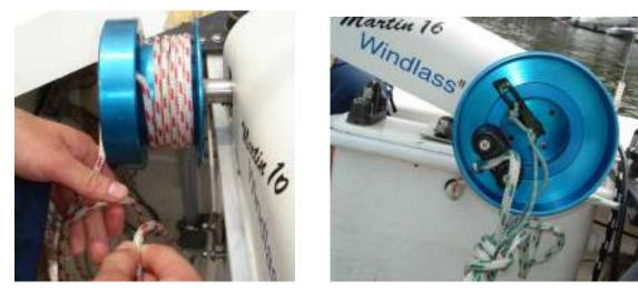
5) Plug the Windlass into the Autohelm. You may need to use the jib fine-tune to assure that the main and jib are in sync (at the same approximate angle to the centerline of the boat). In most Martins the other end of the jib exits at a cleat near the port-side sail controls (by your left elbow).
