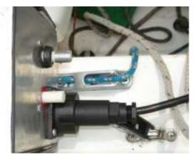
For the "sip n' puff" system, the straws plug into the two white extremities at the front of the autohelm. The picture above illustrates the two white extremities. Some boats use an external sip n' puff connector, which is simply a small box with similar connections.
