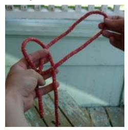
Step 4: Wrap the end of the rope around the main rope.
