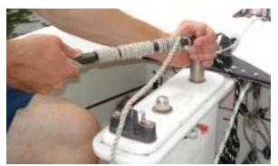
2) Slip the back of the windlass (metal slotted plate) in between the washer and the bolt.
