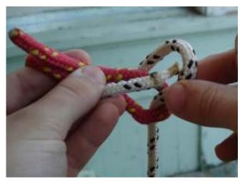
Step 5: Hold on to both pieces of the thick rope loop and the ends of the thinner rope and pull.
