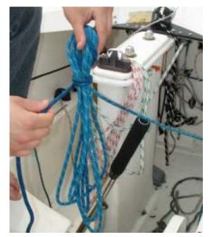
2) When there is not much rope left to coil, you start rolling the rope around the loop you have formed.
