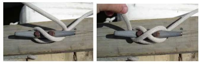
Step 3: Now comes the tricky part. To make sure that the painter stays securely tied to the horn cleat, you must keep crossing it from one "horn" to the next but this time you must make a loop out of the painter before putting it around the "horn". Look carefully the image below.
