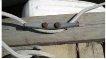
Step 2: Take the end of the painter and start passing it around the "horns" of the horn cleat by crossing it from left to right and right to left.
