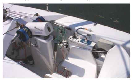
Amazingly, the boat can be even further adapted: the autohelm can be controlled by a straw system called the "sip n' puff". As the name indicates, instead of controlling the helm and sails with hands, the sailor uses their breath. By just inhaling or exhaling gently into the straws, the rudder will move left or right and the sails can be let out or drawn in. With this amazing design, high-level quadriplegics - those with *no* movement below the neck - can independently sail the boat.
