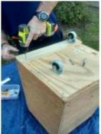
2 Transfer Boxes cut from one– 4' x 8' sheet of 1/2" cabinet grade plywood
