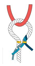
Flip the entire piece of rope over. You have one working strand left to tuck, and there is one strand left in the standing part of the rope that doesn't have a working strand under it. Make this tuck, continuing to work counter to the lay, or twist, of the rope. Mark with a 3.
