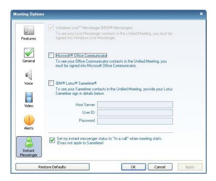
4 To integrate with Lotus Sametime, check the corresponding box and enter your host name, communication port, user ID and password. Click **OK** to save the setting.
