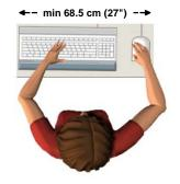
Figure 7: Functional Width Required
