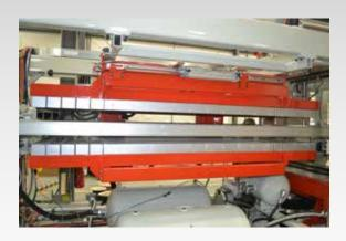
Oven is four times the index length of the forming area and incorporates high efficiency heaters
