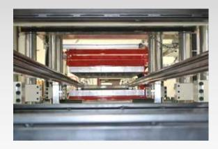
Extra length between forming and cutting stations to allow sufficient cooling when processing PP
