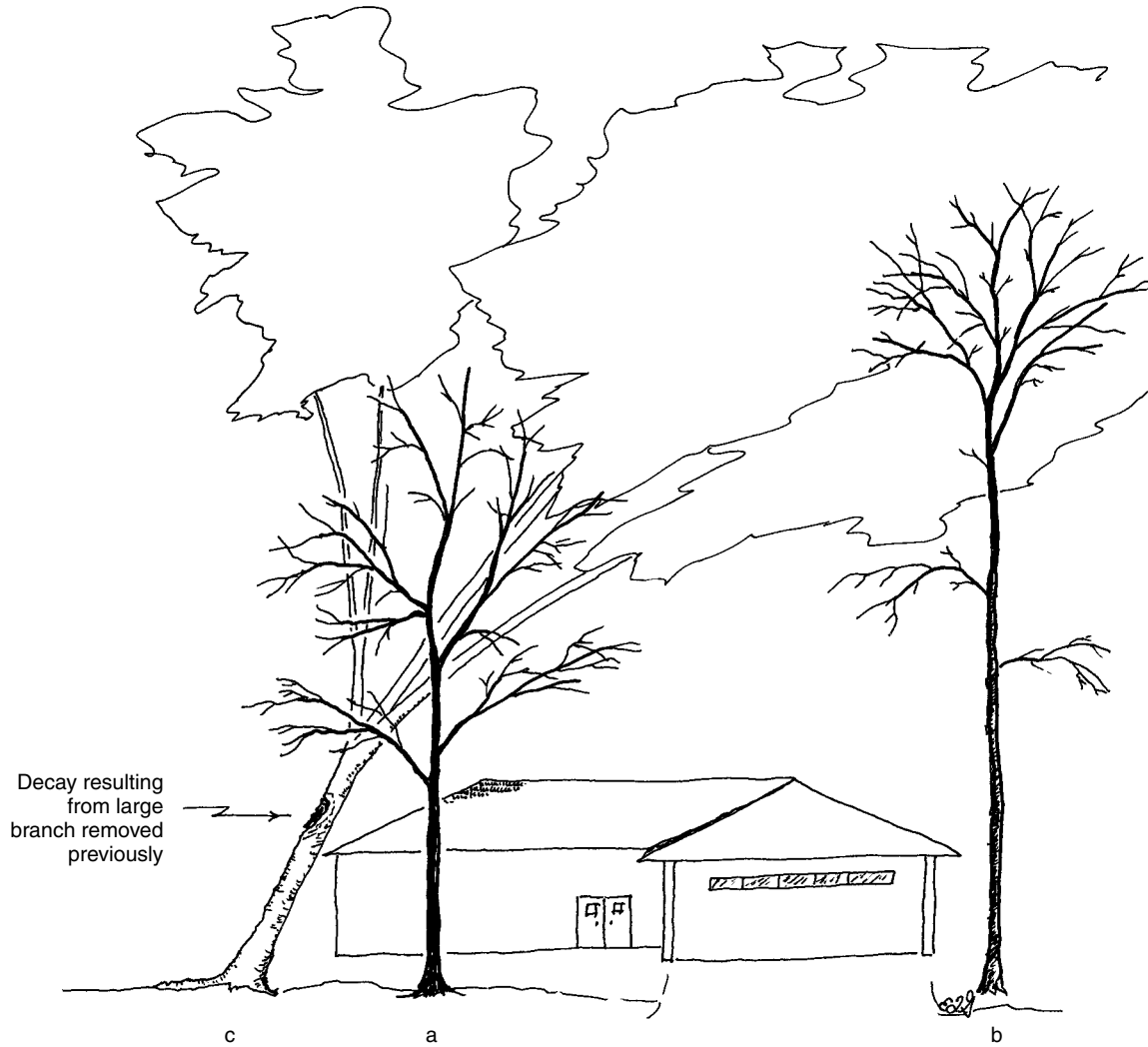
FIGURE 2-9. *Tree 'a' is most suited for saving because: 1) large trees are tough to save—smaller ones, like this one, do best. 2) small trees recover from root damage best. 3) there is one trunk and well spaced branches. 4) there is no included bark or other defects in the branch union. 5) the trunk is straight up. *Tree 'b' is OK but not a great tree because: 1) its very tall with most branches only at the top 2) the trunk is thin-tree may bend over or blow over if nearby trees are removed. *Tree 'c' is poorly suited to save because 1) large trees are tough to keep alive after roots are damage during construction 2) tree is leaning badly 3) trunk forks in the bottom half of the tree 4) tree hangs over the house 5) there is included bark in the bark unions 6) the trunk is decayed at the point where tree was pruned years ago 7) most foliage is toward the top of tree.
