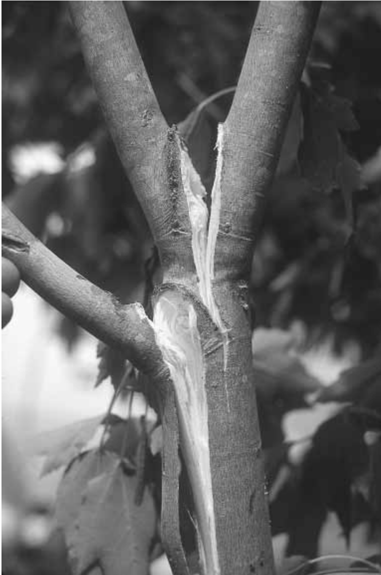
FIGURE 3-7. A small diameter branch (lower union) attached to a much larger trunk is better secured to a tree than a codominant (upper union). Twice as much load (56 kg) was required to split the small branch from the trunk than to separate the upper codominant stems (27 kg).
