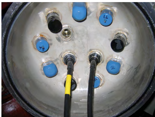
Figure 2.4. Lid of the SNOMS flow through tank loaded with the nine Aanderaa sensors ready for operation.
