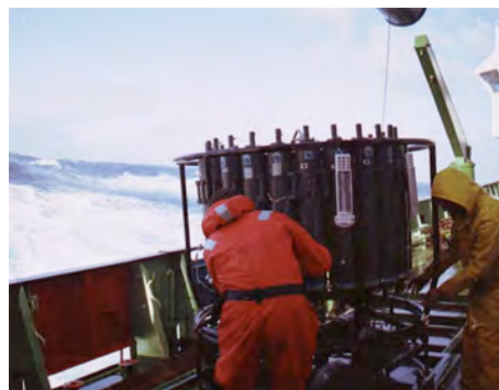
Figures 4.3 and 4.4. Above sampling water from the water collecting bottle on board HMS Challenger in 1874. Below sampling water form the a 24 bottle “rosette” on RRS Discovery in 2012.
