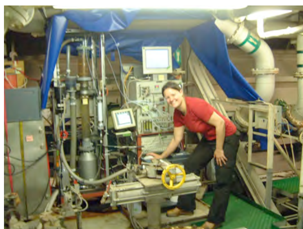
Figure 4.5 An underway system for measuring p\text{CO}_2 in surface seawater. Seen on board MV Falstaff in 2002 operated by IfM Kiel, Germany, designed and built by JAMSTEC Japan.
