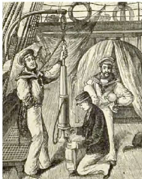
Figures 4.3 and 4.4. Above sampling water from the water collecting bottle on board HMS Challenger in 1874. Below sampling water form the a 24 bottle “rosette” on RRS Discovery in 2012.
