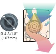
Large cross flow fan – A new and improved fan design delivers higher performance with lower energy consumption and whisper-quiet operation as low as 19 dB(A). Greater airflow up to 453 CFM delivers greater temperature stability throughout the conditioned space.
